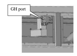
4. Engage the mulching head for 5-10 seconds and record pressure at the GH port.
